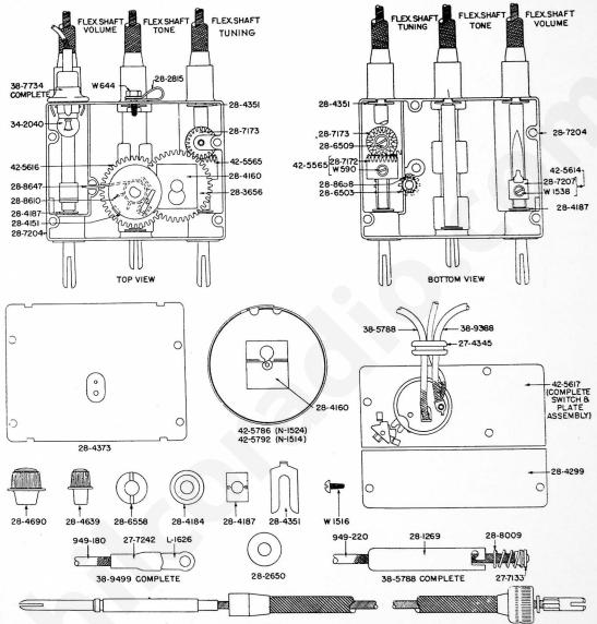
28-8813 TUNING CONTROL SHAFT (N-1524) 28-8815 TUNING CONTROL SHAFT (N-1514)
